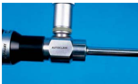
Figure 22. Example of an endoscope with the manufacturer's stamp to certify that it can be autoclaved
